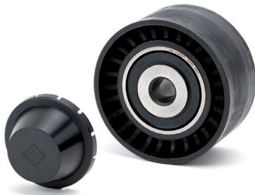
Figure 1: Old design with protective cap
